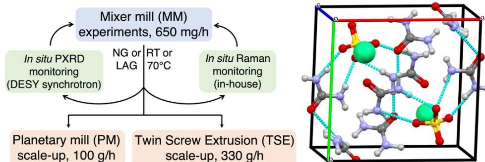
**Figure 1. Reaction scheme for the small and large scale synthesis of calcium urea sulfate (URCASU, the crystal**
